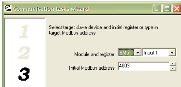
Fig. 16. Assignment to the device and definition of the beginning address.
