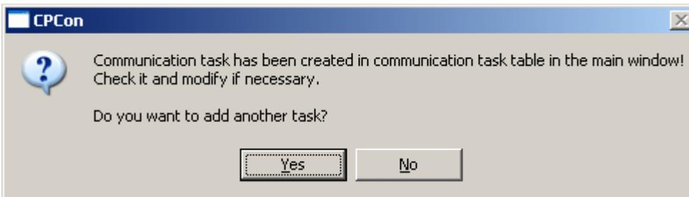
The first line with data set in the creator appears in the table of communication tasks and with it, the conversion of registers into bytes, 16 → 8 bit.
