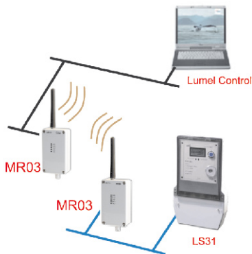
Fig 1. Exemplary remote readout of LS31 watt-hour using the MR03 module
