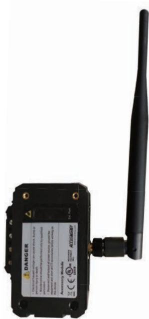
AXM-MESH transceiver module that can only be attached to the Acuvim II series meters.
