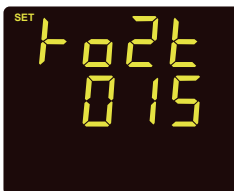
Fig 3-36 RO2 Alarm Delay Setting
