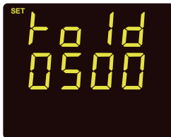
Fig 3-26 RO1 Momentary Delay Time
