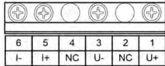
a. Voltage and Current Terminal Strip
