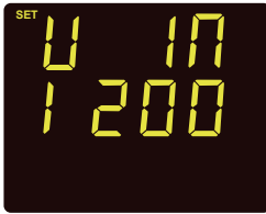
Fig3-6 Range Voltage setting
