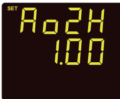
Fig 3-24 AO2 Up Limit Setting
