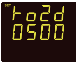
Fig 3-32 RO2 Momentary Delay Time
