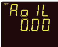
Fig 3-20 AO1 Lower Limit Setting
