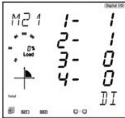
Figure 5-17 Digital Status Reading from Acuvim II Display
