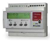
EDS (Efficiency Data Server) is an energy efficiency manager. The device has an RS-485 communications bus, as well as 8 digital inputs and 6 digital outputs via relay, which allow it to communicate with external field devices, representing and storing the information via its Ethernet connection and integrated web server. EDS also has a standard XML server, through which other external applications can integrate information from the device easily and intuitively.
