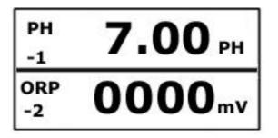
Note: Under main interface through press " , shift to CH-1 browsing interface, press " To shift to browsing CH-2 browing interface, no need to enter 'Menu Option' interface, it could browse setting value.
