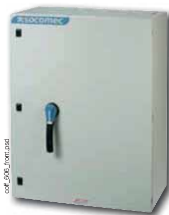
FUSERBLOC enclosure 100 to 800A Painted steel - IP65
